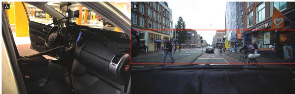
Figure 2. Recording and editing of traffic scenes. A. The car and camera setup. B. Indication of crop to 5760 × 1200. The full width of the video was used. No information about the traffic scene was lost by cropping the video's height to facilitate screen fitting.
