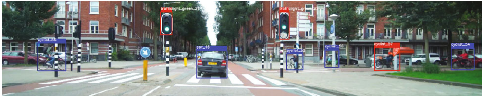
Figure 8. A snapshot of a traffic scene with areas of interest highlighted with rectangles, including five cyclists, one car and two traffic lights. The red rectangles denote “Must-Be-Seen” objects, signifying objects that demand active or passive consideration by the driver, provoking actions like speed reduction, lane change, or delayed acceleration. The blue rectangles represent “May- Be-Seen” objects, which are relevant to be seen by the driver, but do not necessitate a change in driving behavior, such as pedestrians on the sidewalk and oncoming traffic in the other lane. In this depicted scene, one cyclist is classified as a Must-Be-Seen object due to an upcoming situation where the cyclist approaches to cross the road.
